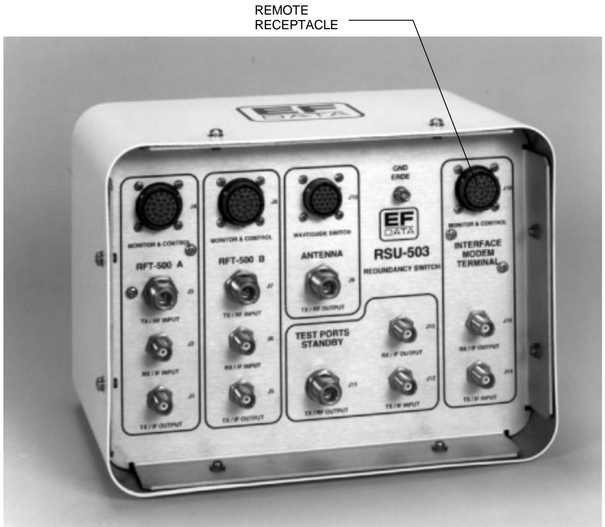
Figure 4. RSU-503 External Connections
